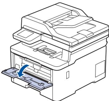
3. Use both hands to slide the manual feed slot paper guides to fit the width of the paper you are using.
