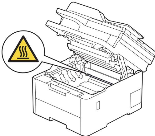
3. Remove all of the toner cartridge and drum unit assemblies.
