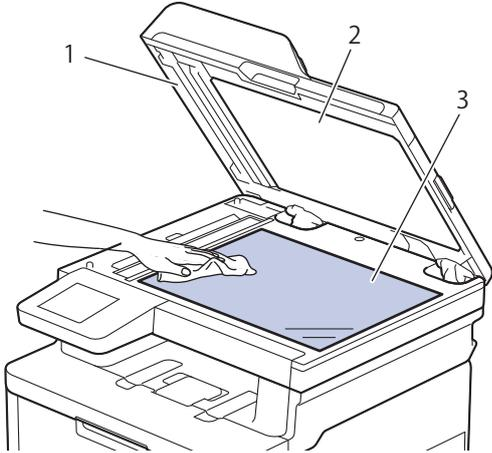
3. In the ADF unit, clean the white bar (1) and the scanner glass strip (2) underneath it with a soft lint-free cloth moistened with water.
