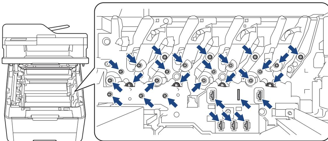
3. Clean the corona wire inside the drum unit by gently sliding the green tab from left to right and right to left several times.
