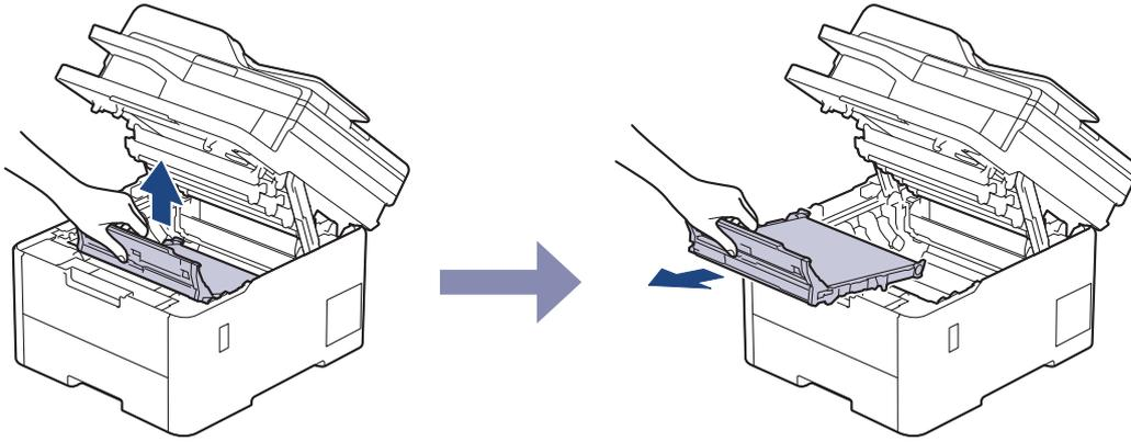
5. Unpack the new belt unit and insert it into the machine.
