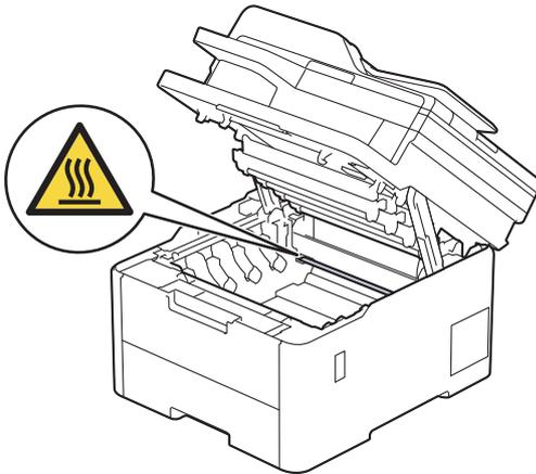
3. Remove all of the toner cartridge and drum unit assemblies.
