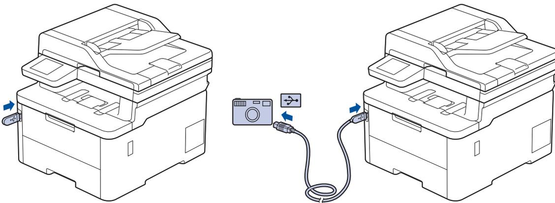
1. Connect your USB flash drive or digital camera to the USB direct interface. The touchscreen will automatically display the USB menu to confirm that the USB flash drive or digital camera is correctly connected.
