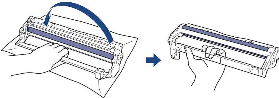
9. Loosen your grip so the frame drops forward, and then use your right hand to locate the drum unit gear inside the right side of the frame.
